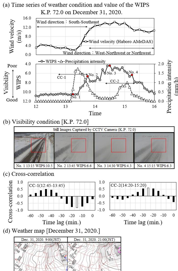
Fig. 7 Time series of weather and visibility conditions at K.P. 72.0 on December 31, 2020.
