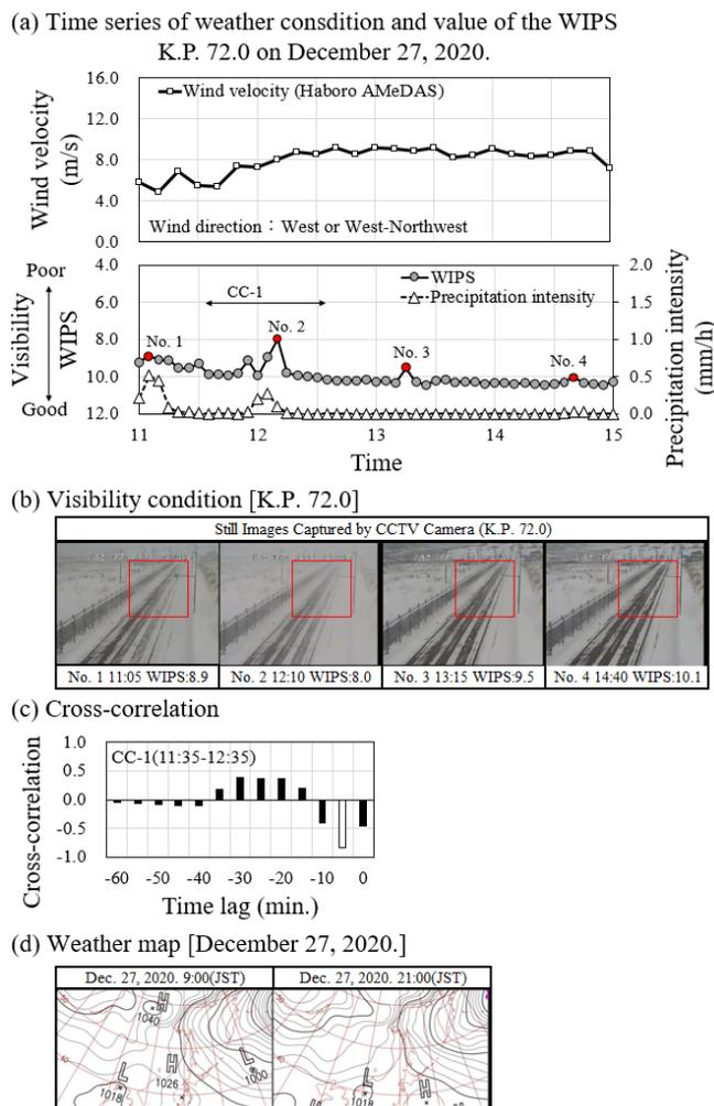
Fig. 5 Time series of weather and visibility conditions at K.P. 72.0 on December 27, 2020.
