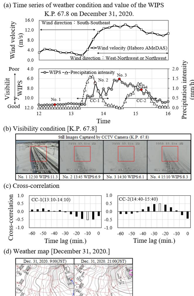
Fig. 6 Time series of weather and visibility conditions at K.P. 67.8 on December 31, 2020.
