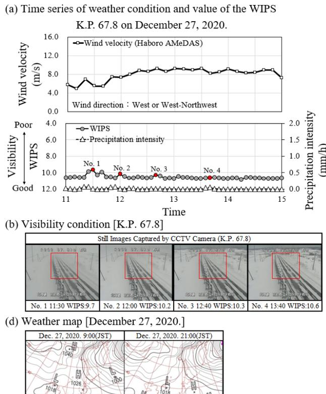
Fig. 4 Time series of weather and visibility conditions at K.P. 67.8 on December 27, 2020.
