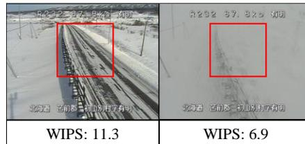
Fig. 3 Values of the WIPS and visibility conditions
